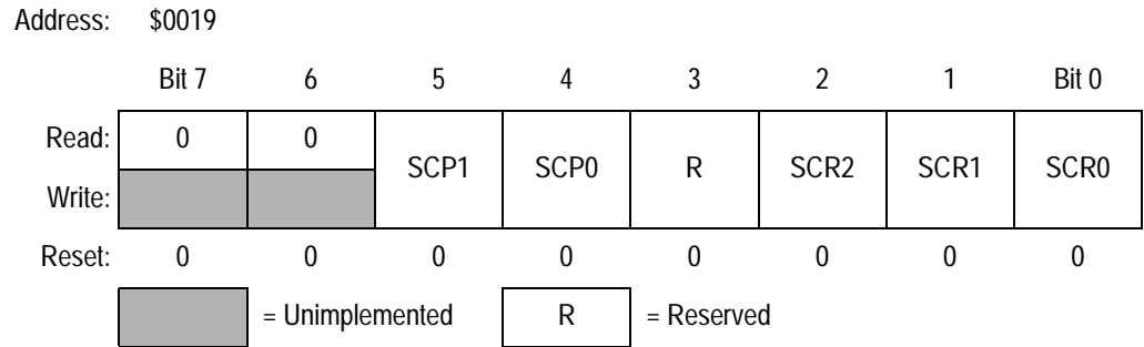
Figure 16-18. SCI Baud Rate Register (SCBR)
